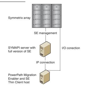
Figure 2 Solutions Enabler Thin Client for Migration Enabler
